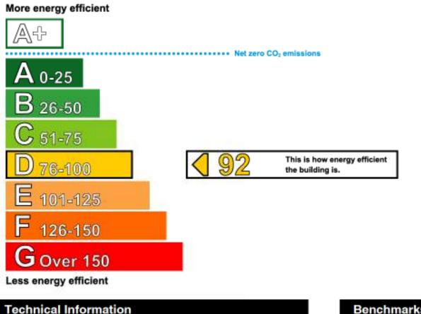
Grid Supplied Electricity Main heating fuel: Building environment: Heating and Natural Ventilation 170 Total useful floor area (m<sup>2</sup>): Building complexity (NOS level): з Building emission rate (kgCO<sub>2</sub>/m<sup>2</sup>): 72.2
